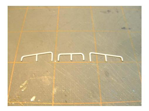
**10.** Also use the template to build these additional gun stops for the forward deck and hatches.
