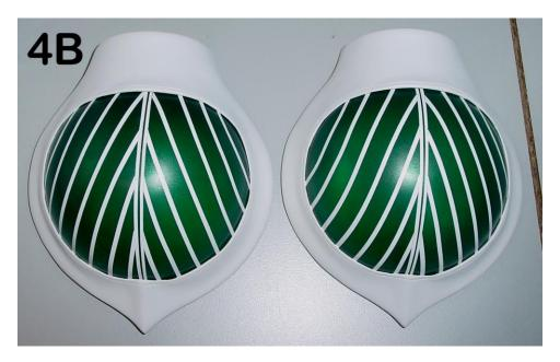
At this point it will probably be necessary to sand the surfaces of the Engine halves that will be glued together to get as smooth a finish as possible. Once the engine halves are glued together it is necessary to fill the joint where the parts meet. This was done in several stages of adding putty followed by sanding. By repeating this process a very nice finish can be achieved, Pic 4C.
