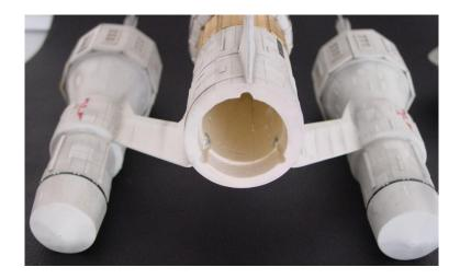
I added three short pieces of brass tubing to the PVC to use as registration points. Corresponding grooves were cut into the wall of the Main Body. Along the way I ensured that the fit was tight so that the parts would stay in place.
