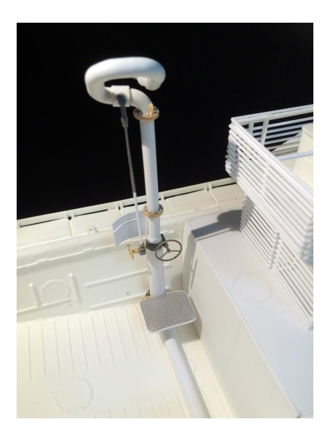
You can start gluing components to the well deck at this point. Work your way back from here to the engine ensuring all the pipes fit.
