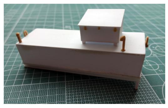
Proper positioning of the fuel tank and gear locker. Do not glue anything to the well deck yet until all the components are assembled.
