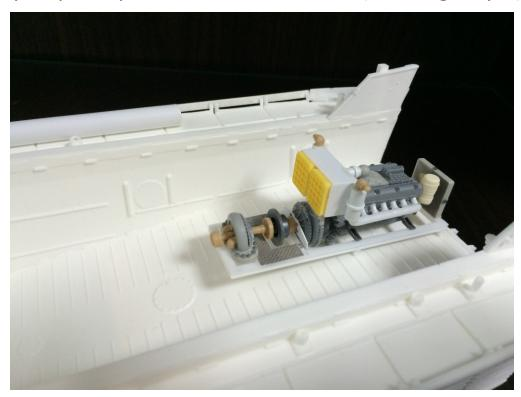
Assemble the centrifugal pump expansion tank and it's support frame.
