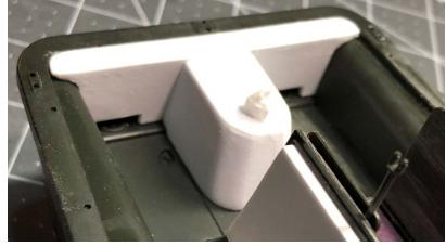
• Install the rope hook in this position on the back of the engine compartment.
