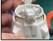
A length of brass rod was used here, so bend and glue in as shown.
