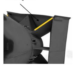
Position center fin support bars (4) made from 1.75" .030 Evergreen Rod on both the Top Center and Bottom Center fins. NOTE: Hole on leading edge of TOP CENTER FIN.
