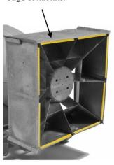
Cut small slice along edge of 1.50" Evergreen Tube (#223) and place on front edge of each diagonal fin.
