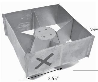
View of outer fins along with center fins, attached to center core.
